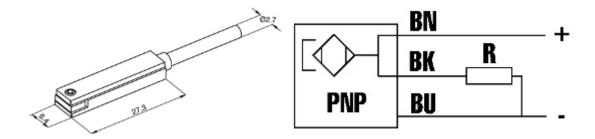
Magnetic switches are electronic detectors, which react in the presence of the magnetic field. Positioned on the cylinder barrel they notice the presence of the magnetic field generated by the magnet assembled on the piston rod. Use on pneumatic systems allows considerably simplifications and it permits an immediate possibility of interface with electrical and electronic circuits.
