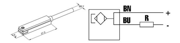
Magnetic switches are electronic detectors, which react in the presence of magnetic field. Positioned on the cylinder barrel they notice the presence of the magnetic field generated by the magnet assembled on the piston rod. Use on pneumatic systems allows considerably simplifications and it permits an immediate possibility of interface with electrical and electronic circuits.
